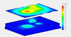
A liquid cold plate, which incorporates turbulators, provides the design engineer much less restriction in size, weight and cost.
