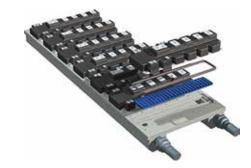
**Die Cast Liquid Cold Plate** is a two piece construction suitable for complex high volume applications. Multiple internal and external features can be incorporated into the two die cast tools. After casting, the two halves can be bonded together by various processes, including welding, brazing or by the use of an epoxy.
