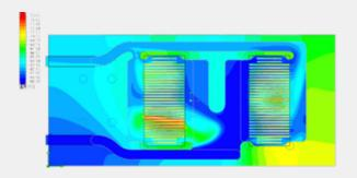
When we develop your cold plates, the design technique for enhancing the heat transfer performance becomes critical. In that regard, consideration is given to manufacturing issues as well as to thermal and fluid flow issues.
