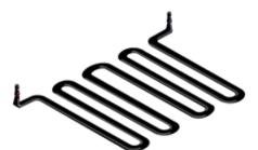
Tube cooler between cells -Serpentine cooler.
